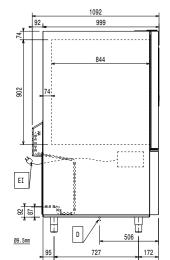
Drain Electrical inlet (power) FΙ Refrigerant Outlet
